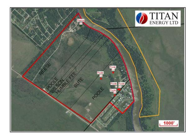
Aerial image of the Allen Dome area that is Titan Energy's focus area, along with current and proposed well locations. The area encircled in red indicates the outline of the Northern and Southern flanks of the salt dome. The ground within the yellow lines on the right hand side is the new "Perry Ranch" lease area.
