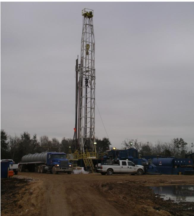
*The Rotary Exploration Rig 2 is currently drilling the Reese #10 exploration well at the Allen Dome North field in Texas. Water from recent heavy rains is still visible in the right foreground.*
