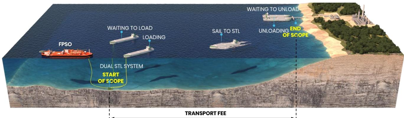
Figure 1 outlines the scope of the Commercialisation Plan. Loading export gas from the FPSO via a dual Submerged Turret Loading (STL) buoy system and transporting using a fleet of CNG Optimum ships to an onshore gas processing facility, located within 200 nautical miles or less than a days sail. The FPSO is to be designed for up to 90,000 Bbl/d of oil and 300 MMscf/d of gas production.
