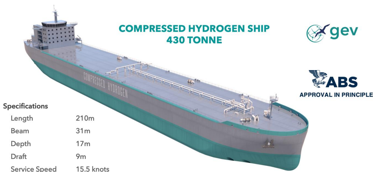
Figure 1: Compressed Hydrogen Ship General Arrangement
